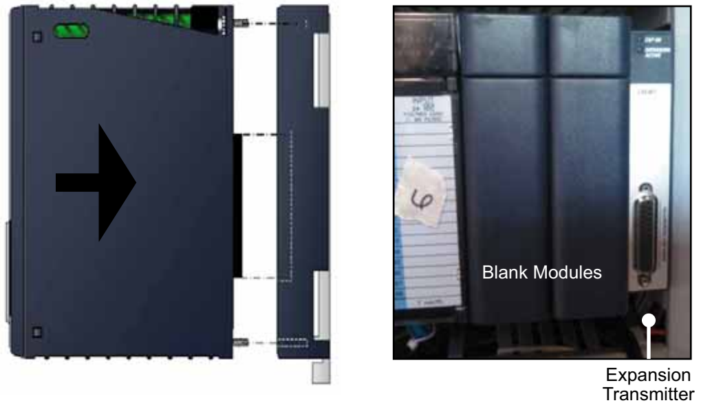
Figure 13: Installing the Expansion Transmitter Module
